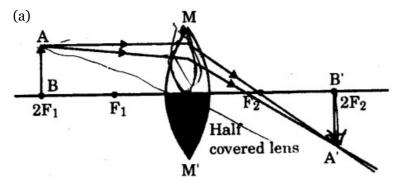
The image is formed at  $2F_2$  and is real and inverted.
